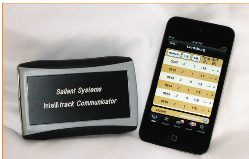
Rail Stress Monitor Hand-held Interrogator™ retrieves stress and temperature data.
